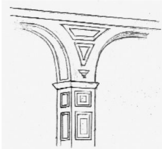
Figure 9.4 A spandrel formed by two designed arches.(Drawing by Celeste Behe.)
