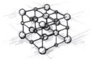
Figure 4.2. Three-dimensional structure of a salt crystal. Sodium atoms are represented by the light-colored balls; the chlorine atoms by the dark-colored balls.
