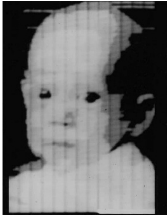
The world's first digitized photo, of Russell Kirsch's son Walden. Made in 1957, it's made of 30,976 black-or-white pixels.
